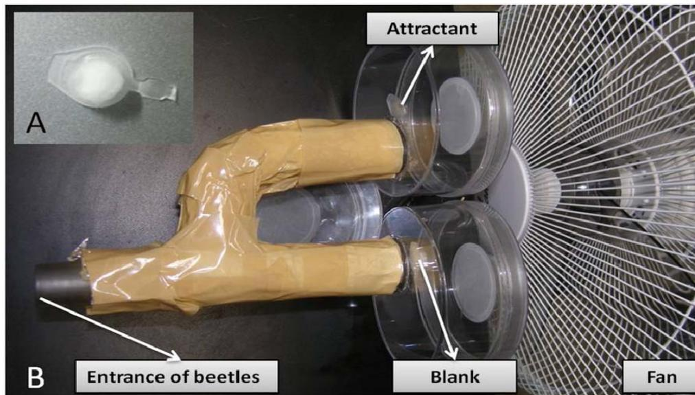
**Fig. 1:** The device used to evaluate the effectiveness of the tested attractants. A, the attractant container; B, the whole device, which consisted of one y-shaped passage, two collection cages, and a fan.
