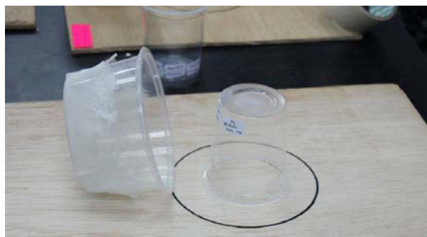
Fig 1: Bed bugs are inserted first before plastic containers with net cloth cover up the treated surface.
