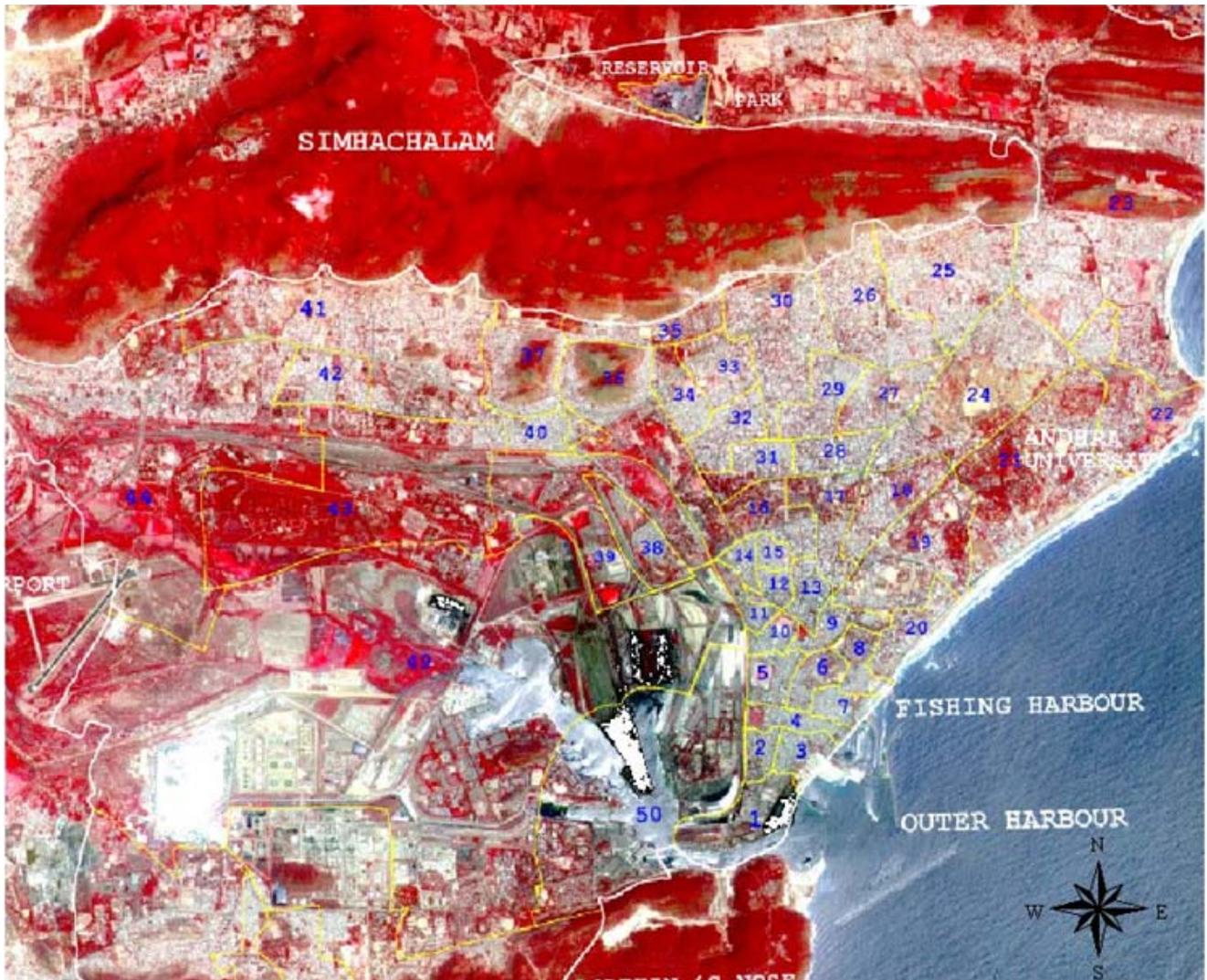
**Fig 2:** Land use/ land cover image of the study area with 5m X 5m resolution is obtained from a systematic value added hybrid colour composite image of the IRS PAN and LISS III with high spatial resolution of 1:25,000
