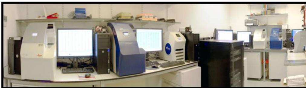
**Fig 1:** A typical arrangement of slide scanners and servers required for full digitization of a laboratory workflow
