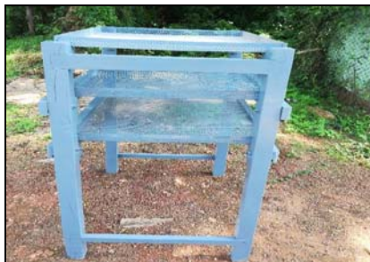
Fig 2: Three tiered perforated tray aerator
