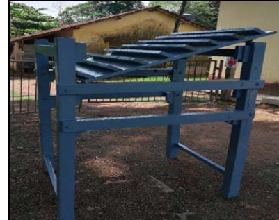
Fig 4: Cascading wooden plank aerator
