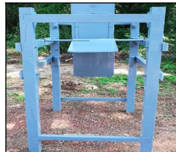
Fig 6: Rotating wheel aerator with stand
