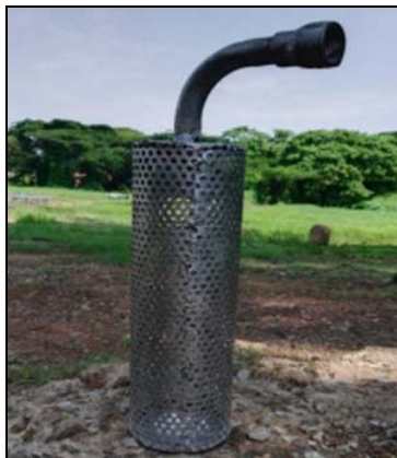
Fig 7: Vertical perforated cylindrical aerator design
