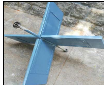
Fig 5: Rotating wheel aerator
