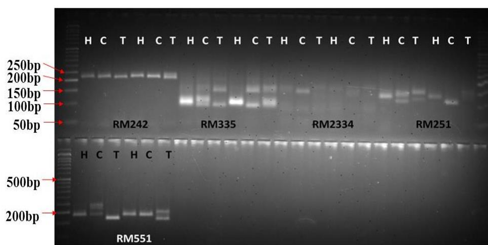
Fig 2: Electrophoregram in 3 rice genotypes using SSR market RM242, RM335, RM2334, RM251 & RM551. In each Lane1: Molecular ladder (50bp); Lane2: Hasanta; Lane3: Resistant check & Lane4:TN1
