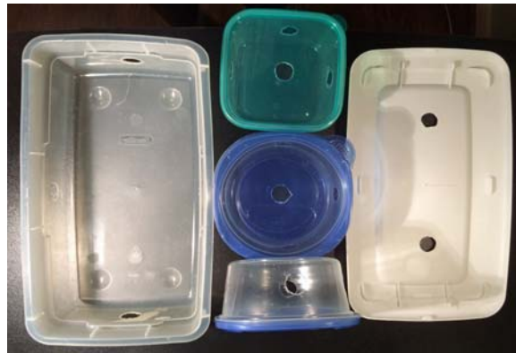
Fig 1B: Minimally vented refrigeration holding containers of varying sizes for ova and pupae
