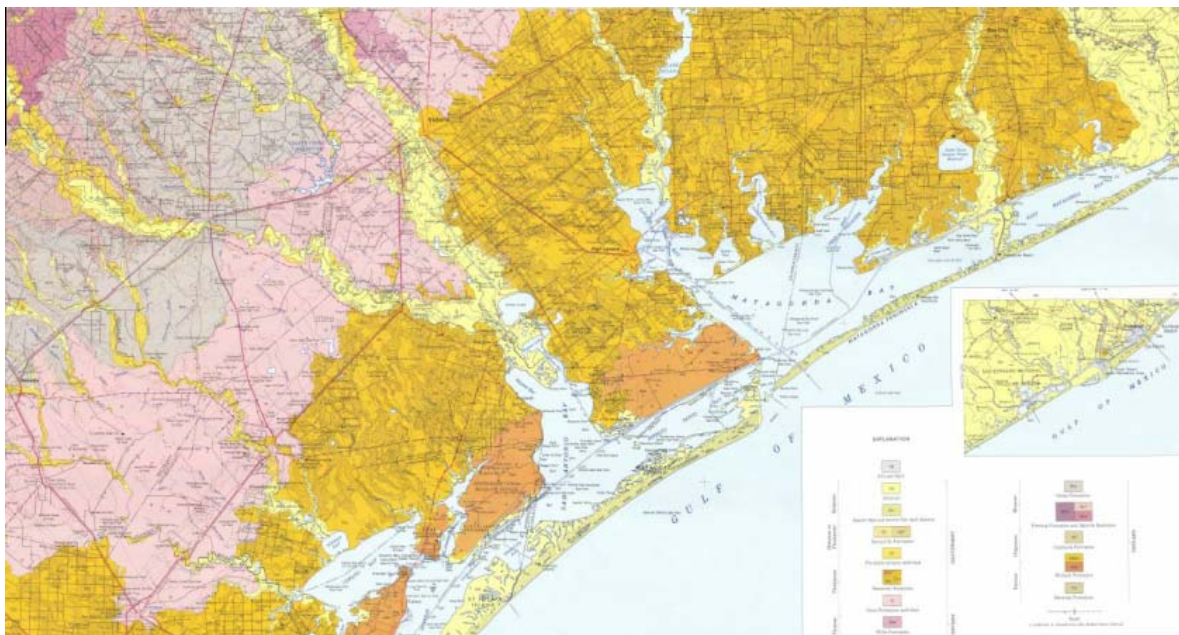
Fig 1: The Geologic Atlas of Texas, Beeville Sheet shows the Ingleside Formation in brown. The coastal edge of Calhoun County and several counties to the South are characterized as Ingleside Formation.
