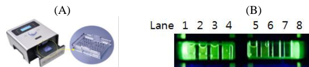
Fig 1: Lab-chip based ultra-fast PCR and lab-chip fluorescence due to SYBR Green.
