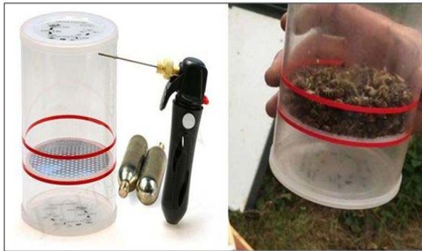
Fig 1: Varroa mite CO 2 spender used for separate the mites from the bees after anesthetize bees with CO 2 gas after 10-20 seconds and CO 2 dosing arrangement with 2×16 gram CO 2 bottles (enough for up to 12 tests and 200 bees from the brood frame).
