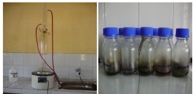
Soxhlet's extraction unit
