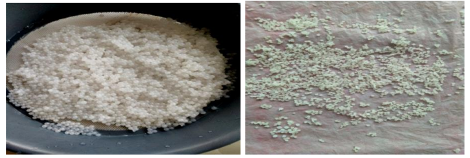
Fig 1: Microcapsules containing different concentrations of eucalyptus oil. 1a. Fresh microcapsules formed after hardening in calcium chloride solution. 1b. Air dried microcapsules used for experimentation.
