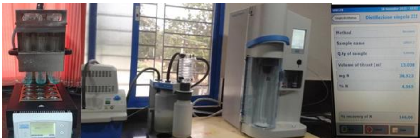
Fig c): Kjeltac auto titration unit for protein estimation
