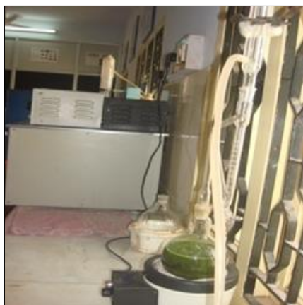
Fig 1: Extraction by Clevenger apparatus
