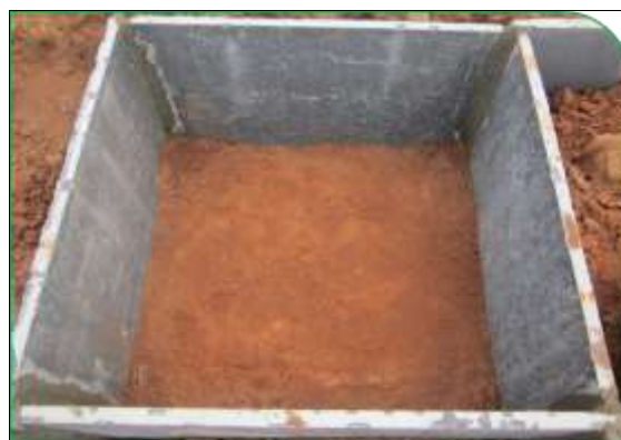
Plate 3: Microplot (1.2 × 1.2 × 0.5 m) built with Kadapa slabs
