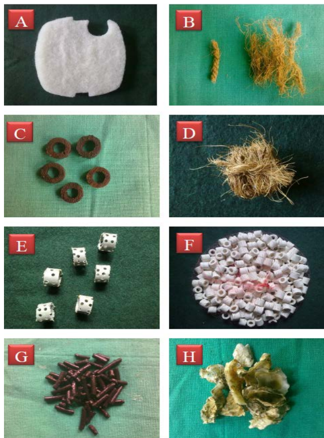
Plate 2: A. Polywool, B. Coir, C. Bamboo rings, D. Bamboo ring + coir, E. Perforated PVC pipe rings, F. Commercial media, G. Activated charcoal, H. Oyster shells
