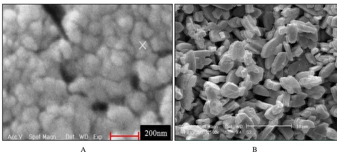
**Fig 1:** The SEM images of synthesized calcium nanoparticles (a) and Calcium macroscales (b)
